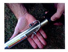
Attach desired implement head (shovel, sledgehammer, axe, or pick-axe) to the Handle-All® assembled handle using the remaining tab lock clevis pin.
