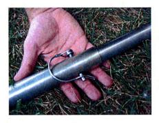
Attach Handle-All® handle pieces together using one of the provided tab lock clevis pins.
