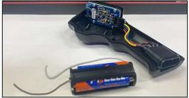
**5.** With battery pack removed, replace the remote control cover and the three screws.
